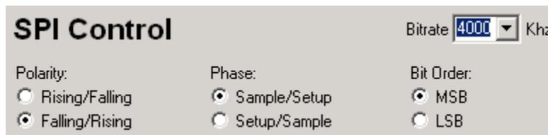
*Figure 14 : SPI Parameters in the SPI Module*
