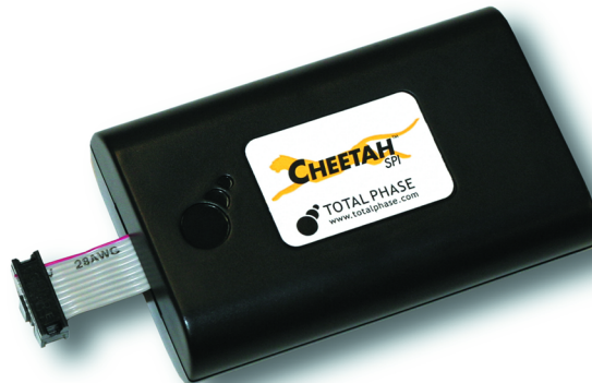
Figure 2: The Cheetah SPI Host Adapter is a high-speed SPI Master-only adapter. It is capable of signaling from 1 to 40+ MHz with no inter-byte delays.
